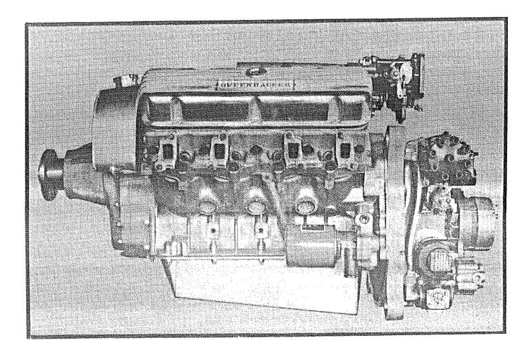
prefer 100/130 Avgas in our engines but the engine is designed for automotive premium so there's no need to burn Avgas unless you plan flight altitudes over 10,000 feet (vapor pressure on auto gas might be a problem over 15,000 feet).
